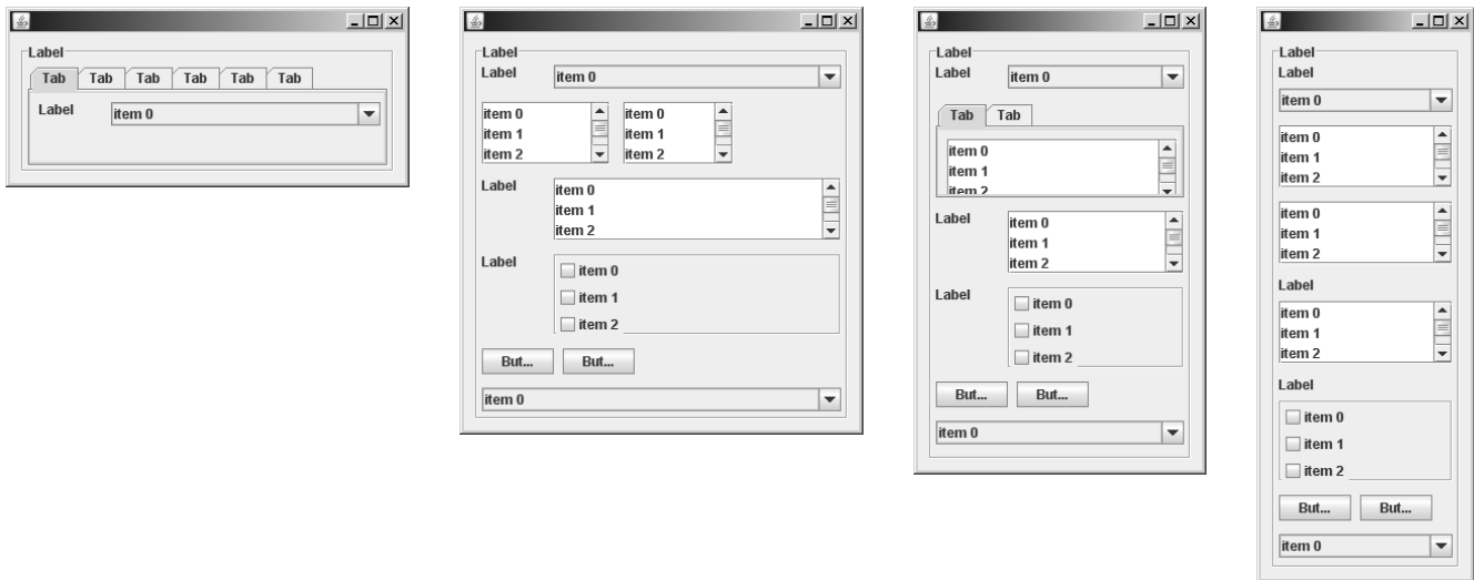
Fig. 5. Results of flexible widget layout from the same UI model with different dialog sizes.
